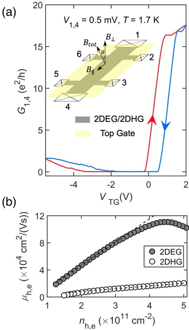
**Figure 3.** (a) Field effect in the Hall bar based on undoped InSb QW. Two-terminal conductance  $G_{1,4}$  measured between contacts 1 and 4 vs. top gate voltage  $V_{TG}$ . The blue and red traces show the down- and up-sweep, respectively. Inset: a schematic diagram of the Hall bar sample and the definition of tilt angle  $\theta$ . (b) The mobilities vs. densities for both 2DHG and 2DEG. The dashed lines are linear fits. Reproduced from [48]. CC BY 4.0.
